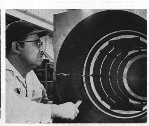
OUTSIDE CORE for a wind tunnel section is prepared by Candelario Torres. Core was made in two sections, baked and assembled. Finished piece weighed more than 1000 lbs. It will withstand tremendous temperatures and strain.
